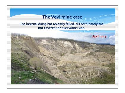
The internal dump has recently failed, but fortunately has not covered the excavation side.
