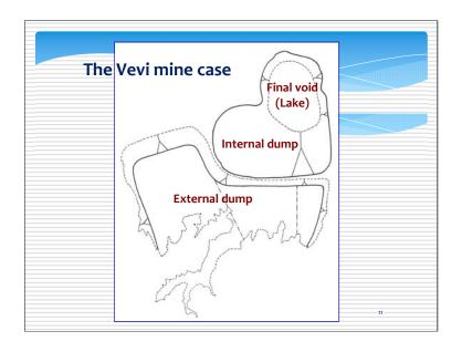
And here is the Life of Mine concept, with the pit limits, the external dump and the internal dump areas with the final void, which is supposed to form a small lake.
