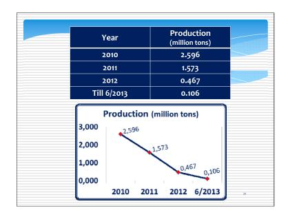
As a result of the narrow pit mining, the limited availability of land and some financing problems, the Achlada mine lignite production fell rapidly from 2.5 million tons in 2010 to 1.5 million tons in 2011 and only 0.4 million tons in 2012. The production in the first semester of 2013 still remains at about 0.1 million tons.
