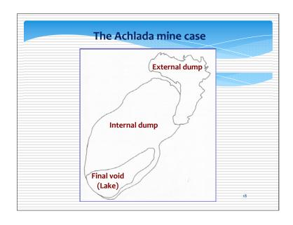
All the waste to be extracted until 2004 should be dumped at an external dump northeast of the pit. After that stage, exclusively internal dumping would be possible.
