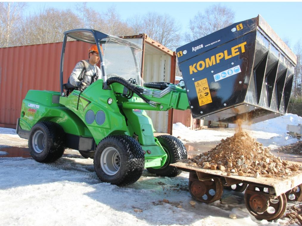
**Crushing with bucket**
