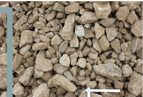
**Limestone for aggregate or backfilling**
