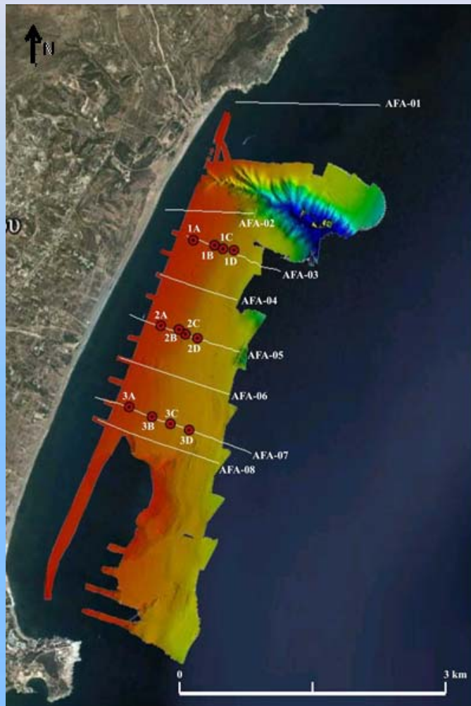
Positions of seismic profiles and of seabed sediments' from Afantou Bay
